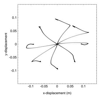
Figure 12: Simulated after-effect trajectories: Hand trajectories for the skeletal dynamics of Eq. (11) in a null force field with the controller of Eq. (12), assuming that the controller had formed an internal model of the force field shown in Fig. 3.
