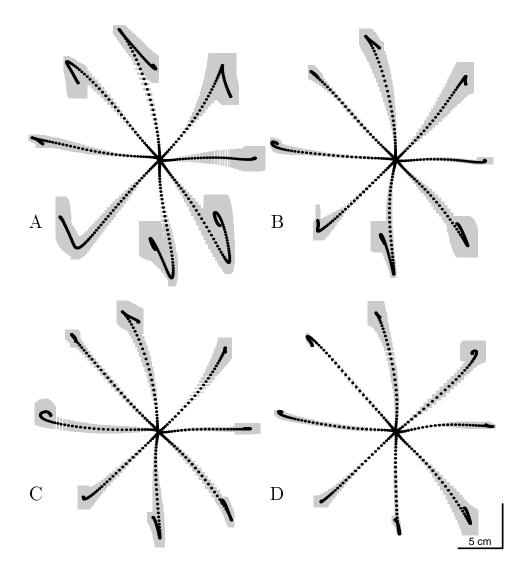
Figure 9: Average  $\pm$  standard-deviation of hand trajectories during the training period in the force field of Fig. 3. Performance plotted during the first, second, third, and final 250 targets (A, B, C, and D, respectively). All trajectories shown are under no-visual feedback condition.
