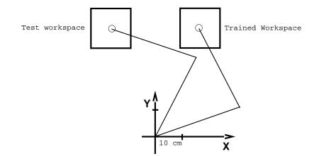
**Figure 2:** Configurations of a model two joint arm, representing typical kinematics of the human arm, at two workspace locations where reaching movements were performed. Typical shoulder and elbow angles at these two workspaces were 15 and 100 degrees at right and 60 and 145 degrees at left, using coordinates defined in Fig. 1.
