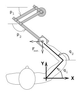
**Figure 1:** Sketch of the manipulandum and the experimental setup. Planar arm movements were made by the subject while grasping the handle of the manipulandum. A monitor, placed directly in front of the subject and above the manipulandum (not shown), displayed the location of the handle as well as targets of reaching movements. The manipulandum had two torque motors at its base which allowed for production of a desired force field.
