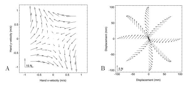
**Figure 3:** An environment as described by the force field in Eq. (1). A: The force field. B: Forces acting on the hand during simulated center-out reaching movements. Movements are simulated as being minimum-jerk with a period of 0.5 sec and amplitude of 10 cm.
