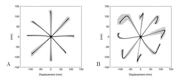
Figure 14: Transferred after-effects: Average  $\pm$  standard-deviation of hand trajectories while moving in a null field at the left workspace. A: Before the subject practiced movements in the field of Fig. 3 at the right workspace. B: After the subject practiced movements in the field of Fig. 3 at the right workspace.
