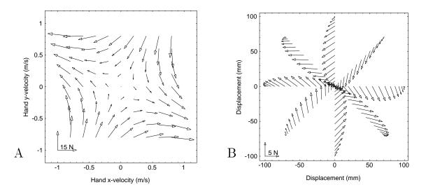
**Figure 4:** An environment described by the field in Eq. (3), plotted as it would appear in the left workspace of Fig. 2. **A:** The force field. **B:** Forces acting on the hand while making reaching movements in the left workspace of Fig. 2 from the center to targets about the circumference of a circle. Movements are simulated as being minimum-jerk with a period of 0.5 sec and amplitude of 10 cm.
