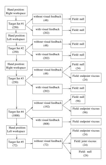
**Figure 5:** Summary of the experimental procedure for subjects in Group 1. The adaptation period was during target set number 4 where an end-point viscous field was present. Subjects in Group 2 underwent an identical procedure except that during the training period a joint-based viscous field was present.
